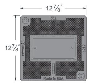
Cover comes standard with permanent markings for manufacturer, load rating, model size and manufacturing location.
