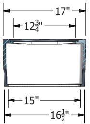
$^{\star}$ Cover comes standard with permanent markings for manufacturer, load rating, model size and manufacturing location.
