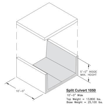
Maximum Inside Height As Shown Can Be Made To Any Height Shorter Than Maximum Designed For HS-20 Loads
