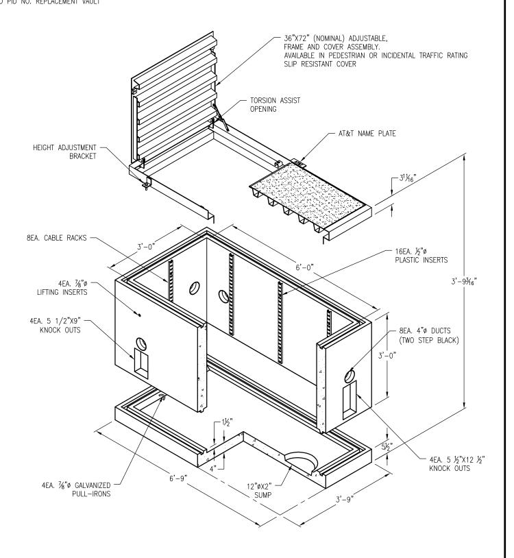
VAULT WEIGHT: 3,380 LBS. FLOOR SLAB WEIGHT: 1,300 LBS.
