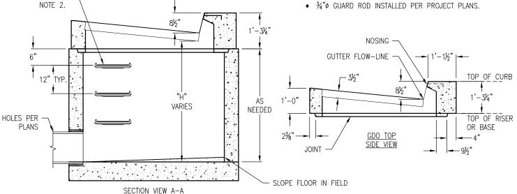
DRAWING MAY NOT CONFORM TO THE MOST CURRENT SPECIFICATION
