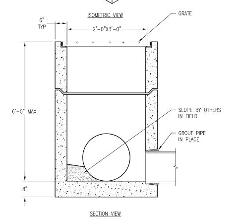
WEIGHT OF FLOOR SLAB IS 1,200 LBS WEIGHT OF WALL IS 900 LBS/FT
