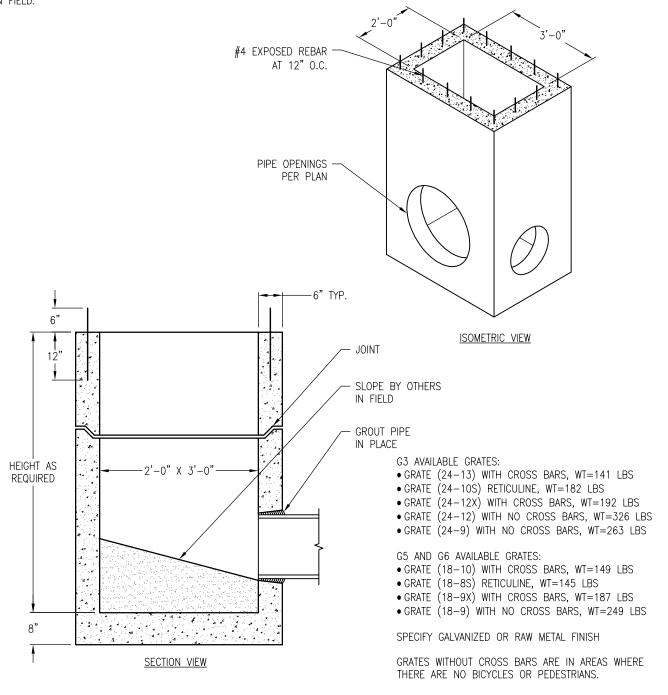
WEIGHT OF FLOOR SLAB = 1,200 LBS WEIGHT OF WALLS = 900 LBS/FT
