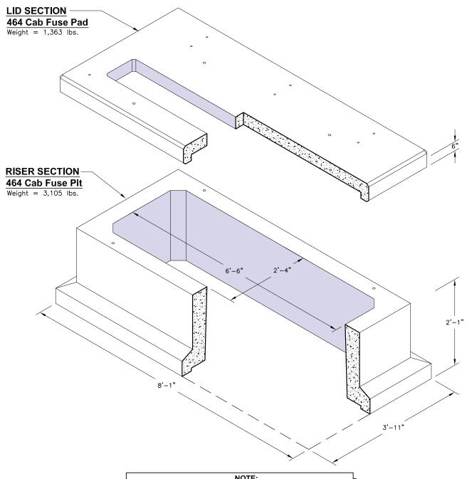
NOTE: Stack Height NOT to Exceed (2) Pit Sections \*Designed for Installation at Grade with Cabinet Loading
