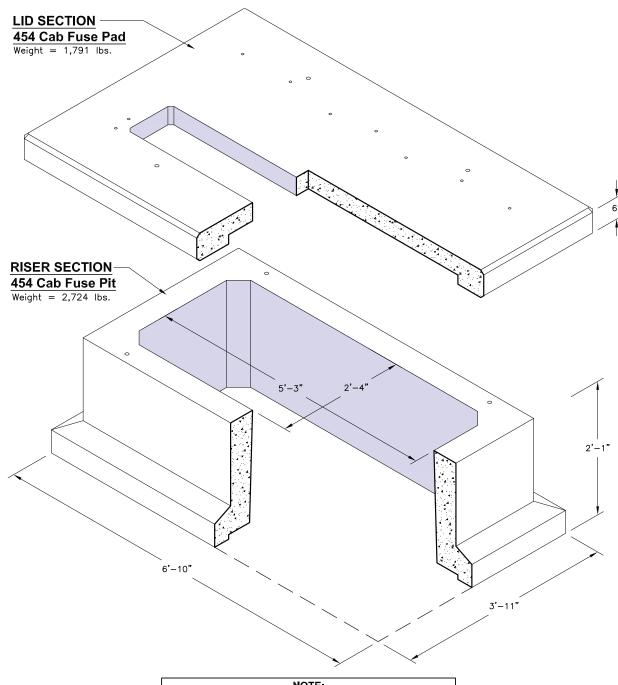
NOTE: Stack Height NOT to Exceed (2) Pit Sections \*Designed for Installation at Grade with Cabinet Loading
