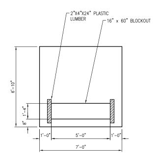
2.4-25 kV, 3-PHASE TRANSFORMER PAD ONLY (NO BASE)
