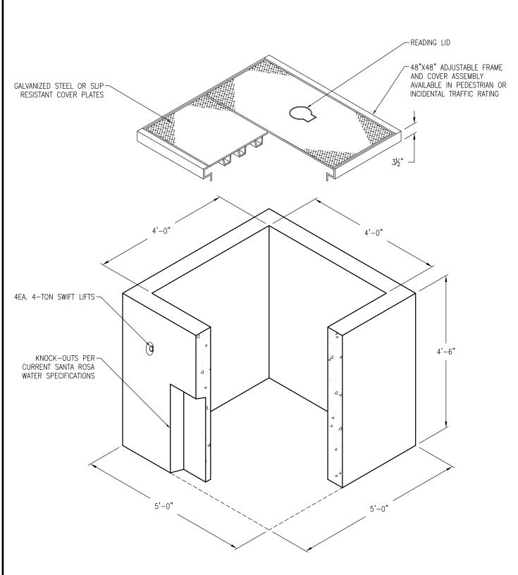
APPROXIMATE WEIGHT: BASE WEIGHT: 6,195 LBS DRAWING MAY NOT CONFORM TO THE MOST CURRENT SPECIFICATION
