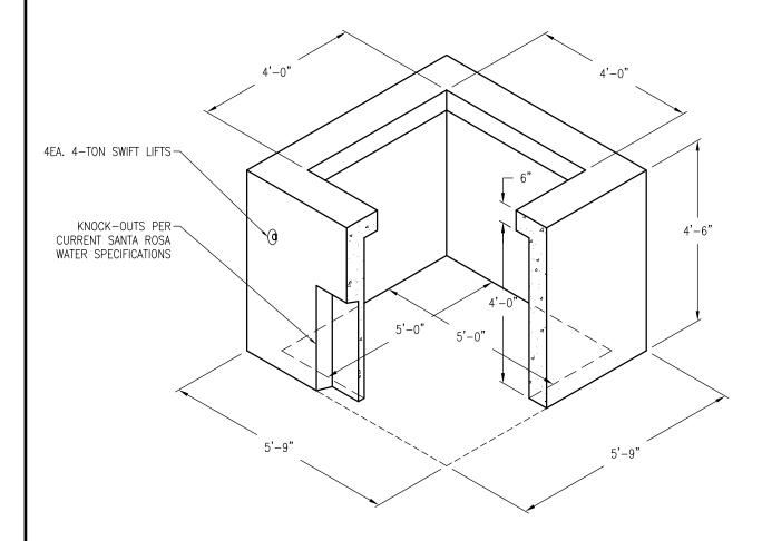
APPROXIMATE WEIGHT: BASE WEIGHT: 7,730 LBS DRAWING MAY NOT CONFORM TO THE MOST CURRENT SPECIFICATION
