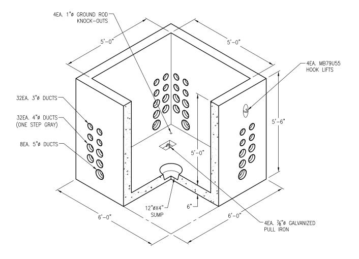
APPROXIMATE WEIGHTS: BASE WEIGHT: 11,170 LBS DRAWING MAY NOT CONFORM TO THE MOST CURRENT SPECIFICATION
