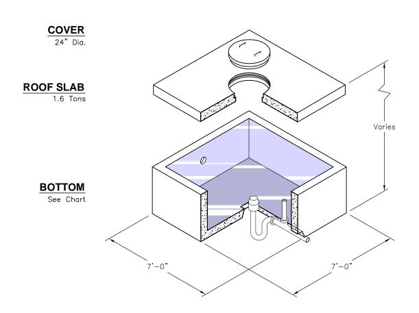
This Siphon Chamber is Available in Single or Double Alternating Models.
