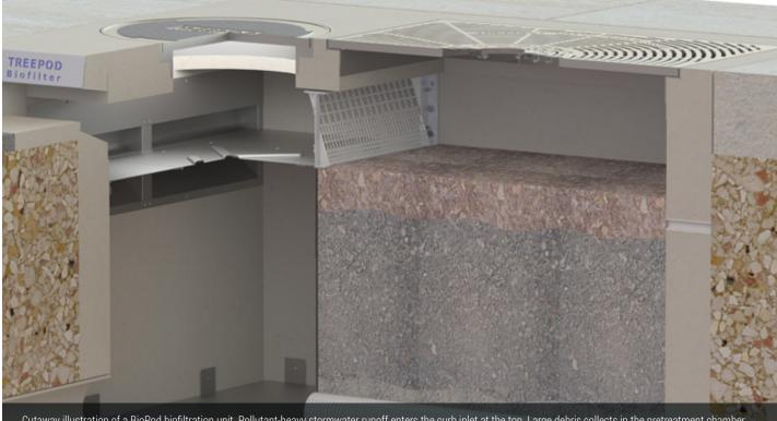
Cutaway illustration of a BioPod biofiltration unit. Pollutant-heavy stormwater runoff enters the curb inlet at the top. Large debris collects in the pretreatment chamber. As water travels downward, pollutants are filtered out by planting media. The tree gets water and nutrients from the collected runoff. Filtered water is collected by the perforated pipe at the bottom and carried out of the unit to the drainage system.
