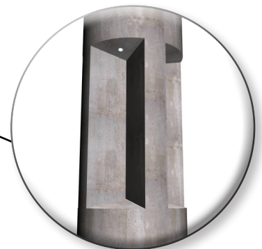
Anti-Rotation Cavities 3' cavities
