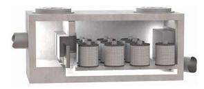
The PerkFilter media filtration system uses physical and chemical treatment processes such as sedimentation, filtration and sorption to remove TSS, metals, nutrients, gross solids, trash, debris as well as petroleum hydrocarbons to significantly reduce the total pollutant discharge load in stormwater runoff. PerkFilter is a media-filled cartridge filtration system where the number and size of the cartridges is tailored to accommodate the water quality flow rate and to
