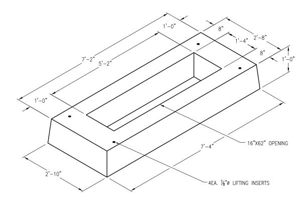
SPPCo PE0025U 3-PHASE PAD JUNCTION ENCLOSURE PAD 2'-8"X7'-2"X1'-0" O.D. PAD 24-0722 PAD WEIGHT: 2,150 LBS.
