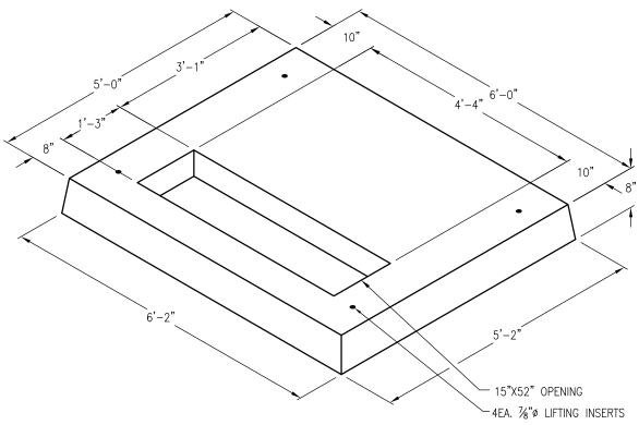
SPPCo PE0003U TRANSFORMER PAD 6'-0"X5'-0"X0'-8" O.D. PAD 24-0697 PAD WEIGHT: 2,700 LBS.
