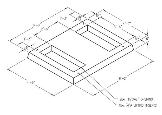
SPPCo PE0012U TRANSFORMER PAD 4'-7"X6'-0"X0'-6" O.D. PAD 24-0726 PAD WEIGHT: 1,550 LBS.
