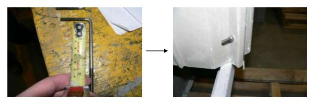
4. Stack the boxes and insert the L-shaped supports through the holes which were intended for the hardware and bolt them to attach the two boxes.
