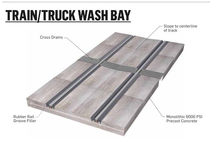
StarTrack precast modules can be customized to provide slope to the center line of track into cross drains, creating easily serviceable Train/Truck-wash stations.
