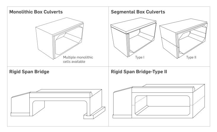
> Factory built precast concrete
