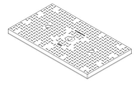
Cover comes standard with permanent markings for manufacturer, load rating, model size and manufacturing location.
