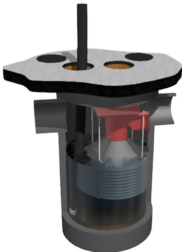
Fig.4 Floatables are removed with a vactor hose .
