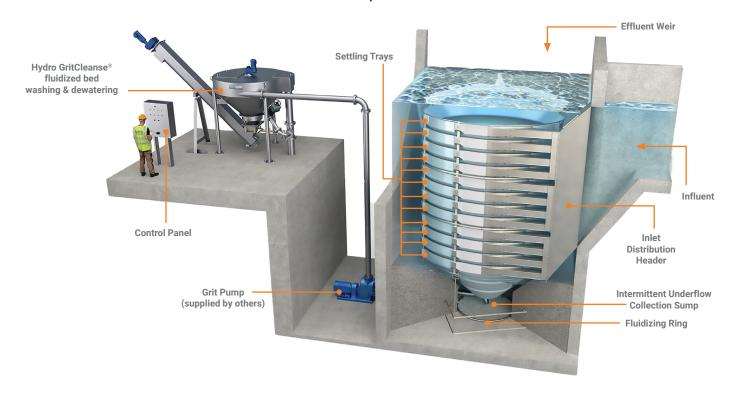
HeadCell<sup>®</sup> Configured for Continuous Operation w/ SlurryCup™ & Grit Snail<sup>®</sup>
